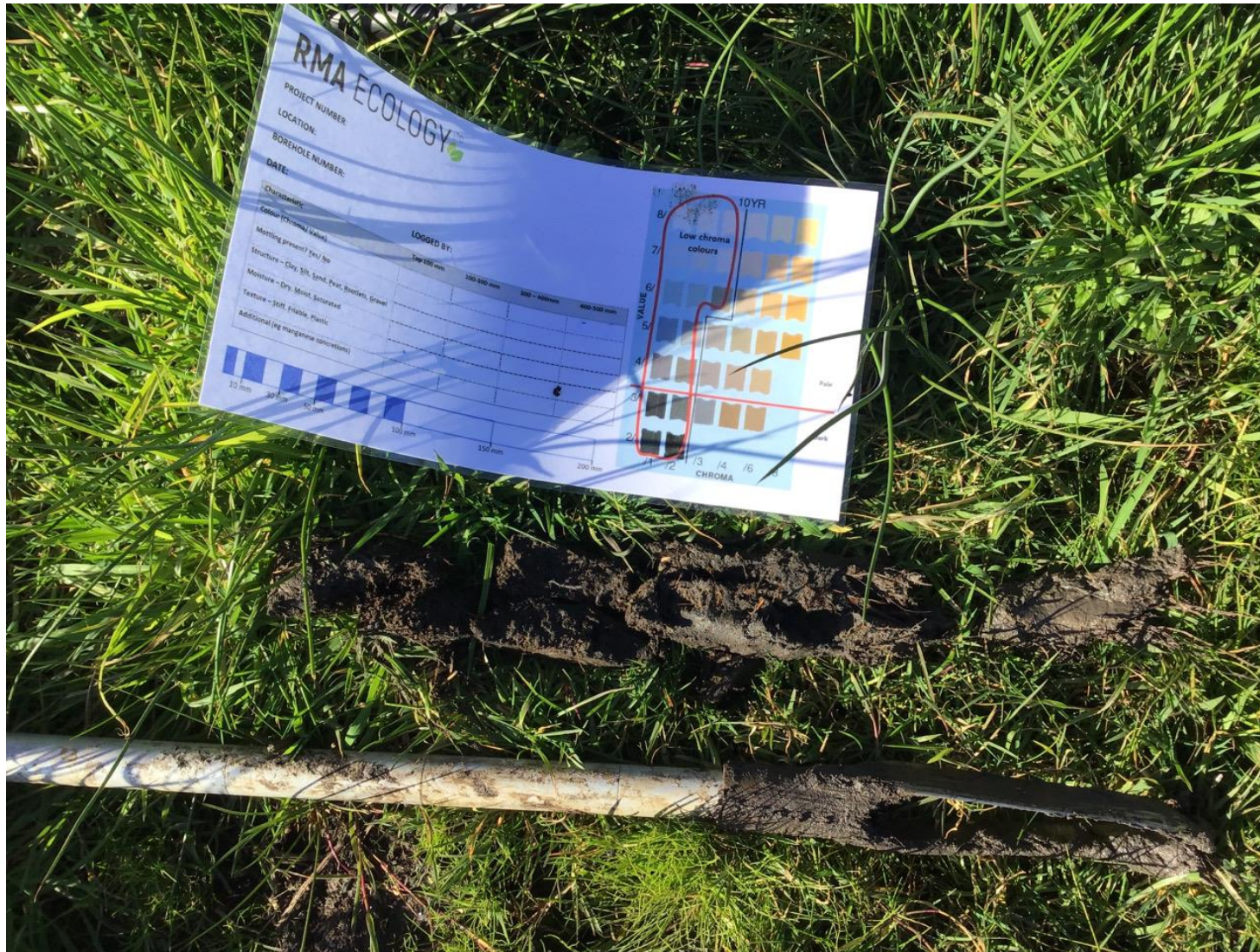
Plate D2. Soil Core W7, an example of a typical low-chroma, saturated wetland soil core which qualifies as a wetland soil.
